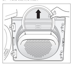
6. Remove the fluff from fine filter. It is best to use a damp hand for this purpose.
